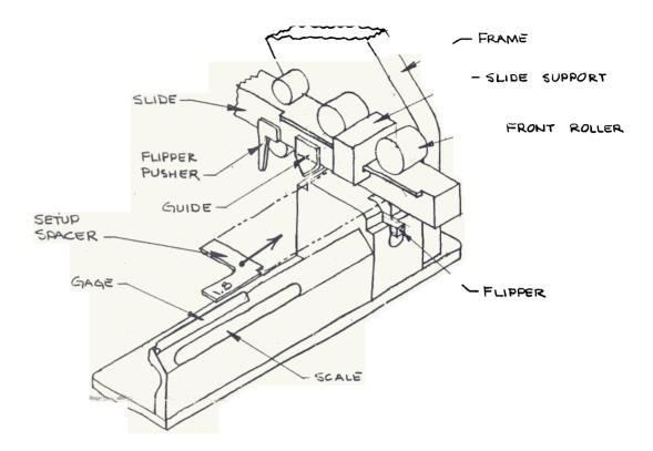
drop out. It will take some practice before you can do this smoothly. If the spokes being cut are oily no further lubrication will be needed. If they are dry a little Tenacious oil should be put on a spoke and the spoke rolled through the machine. This will lubricate the dies sufficiently for threading .75-100 spokes. To cut spokes shorter than 200 mm there is a mark near the left end of the gage that will subtract 100 mm from the scale reading.
