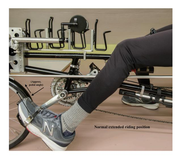
Of course, everyone will have their exact comfort level, but this should get you within about ½" fore or aft. (Don't forget to tighten the steering rod clamp with the front wheel straight and the handlebar at right angles to the frame.)
